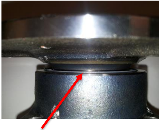
Induced faults on the outer ring and balls
